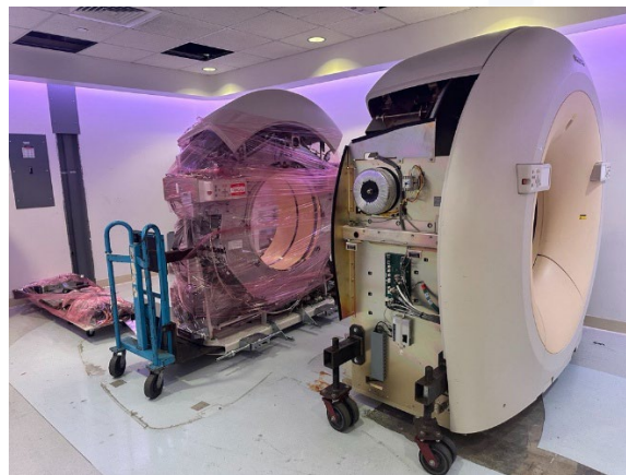
The unit had to be expertly removed in pieces, each of which could weigh around 2 tons.
